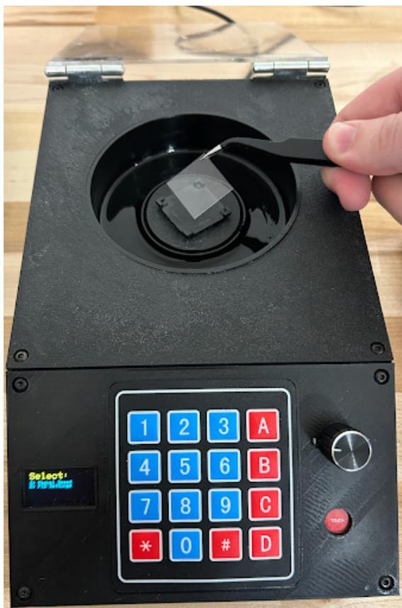
Figure 2.6: Spincoater with a gravity chuck for 22mm glass slides
