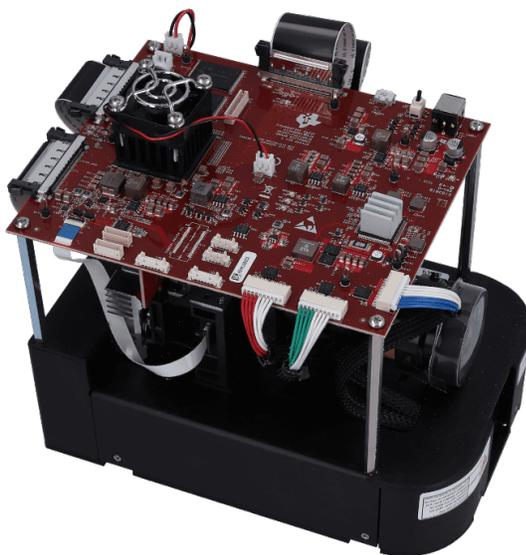
Figure 2.1: Texas Instruments DLP471TP Evaluation Module [16]
